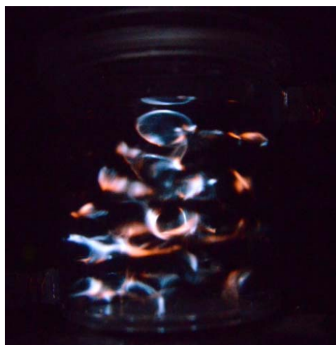
Fig.3 Sonoluminescence from aqueous solution of \text{CaCl}_2 at 71.5 kHz.
