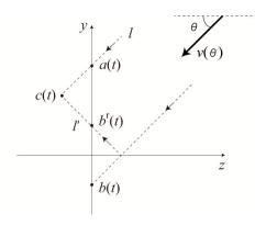
Figure 4: Computation of space curve c(t) from the pair of planar curves a(t) and b(t) on the xy plane.
