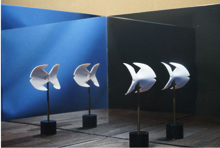
Figure 5. Object creating an anomalous U-turn in the left mirror and an anomalous translation in the right mirror.
