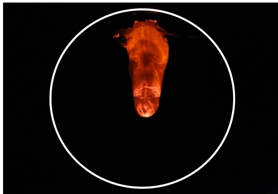
Fig.3 Triboluminescence from Ne induced by the contact of mercury with quartz glass.
