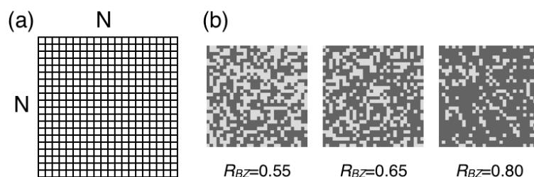
FIGURE 3.22. Schematic illustration of the setting on excitable region in Figure 3.21(C). (a) N \times N square lattice. (b) Examples of image figures varying the ratio, R_{BZ} = 0.55 (left), 0.65 (middle), and 0.80 (right), respectively.
