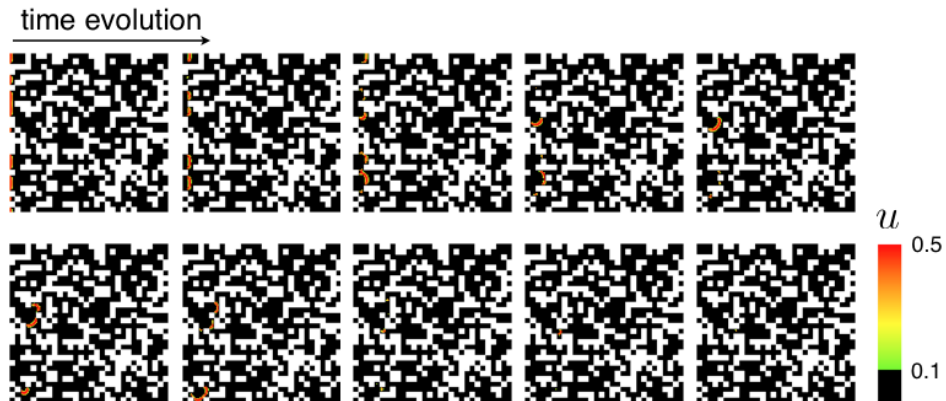
FIGURE 3.31. Chronological snapshots every 1.25 s of the blocked wave propagation state in the case of R = 0.64 . An oxidation wave generated at the left cannot propagate to the right hand side.
