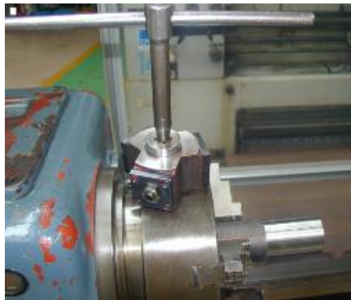
Fig.6 Measuring system for chucking force.
