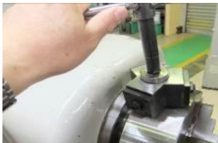
(b) Replacing the jig.
