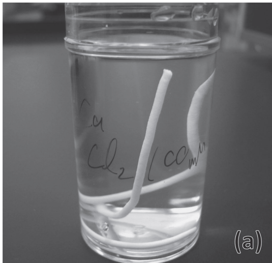
Fig. 2-2 (a) Ca-HAp/Col paste just after injected into 100mM CaCl 2 solution. (b) Ca-HAp/Col paste after immersed 100mM CaCl 2 solution for 1 min.
