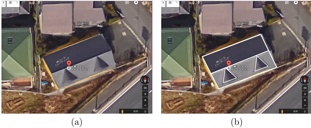
Figure 7.4: Polygon matching of the best ceiling in satellite image. (a) Original image. (b) Matching of the best ceiling
