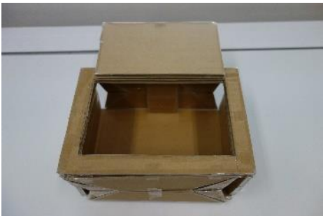
Figure.1.17 A model of a box with thickness which was made of cardboard.
