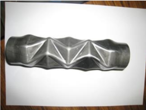
Figure.4.10 RSC of steel material made by hydroforming manufacture.
